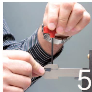
... push the insert onto the contact faces to the stop and fix it in place with the clamping screw.
