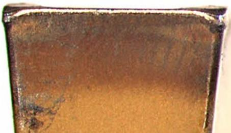
High machining temperature and simultaneous mechanical stress may lead to plastic deformation.
