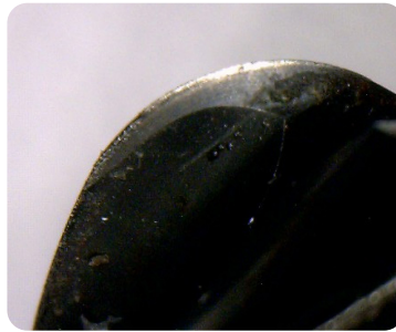
Close up of tool wear
